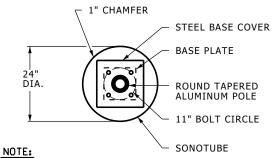
ALL LOCATIONS AND DIMENSIONS FOR ANCHOR BOLTS ETC. SHALL BE VERIFIED IN FIELD BY INSTALLING CONTRACTOR WITH BOLTS AS FURNISHED BY POLE MANUFACTURER.
